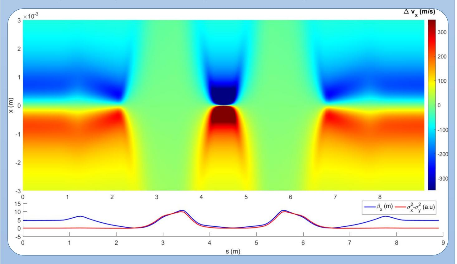
• Color map of the longitudinal kick  $\Delta v_s$  vs horizontal position x and longitudinal position s along half ThomX ring:
