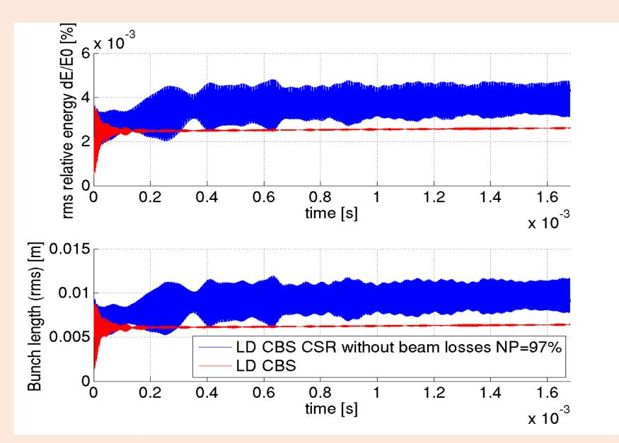
Oscillations of rms relative energy spread and longitudinal bunch length of the electron beam in case of destructive effect of CSR wake field (blue) with simulations made without collective effect (red). Oscillations of rms relative energy spread and longitudinal bunch length of the electron beam with simulation effect of CSR wake field (red) with simulations made without collective effect (red).
