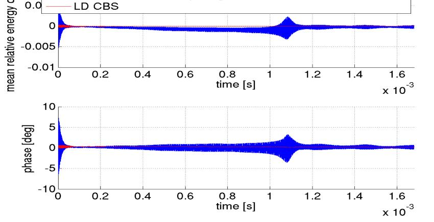
Oscillations of mean relative energy spread and phase of the electron beam in case of destructive effect of CSR wake field(blue) with simulations made without collective effect (red).
