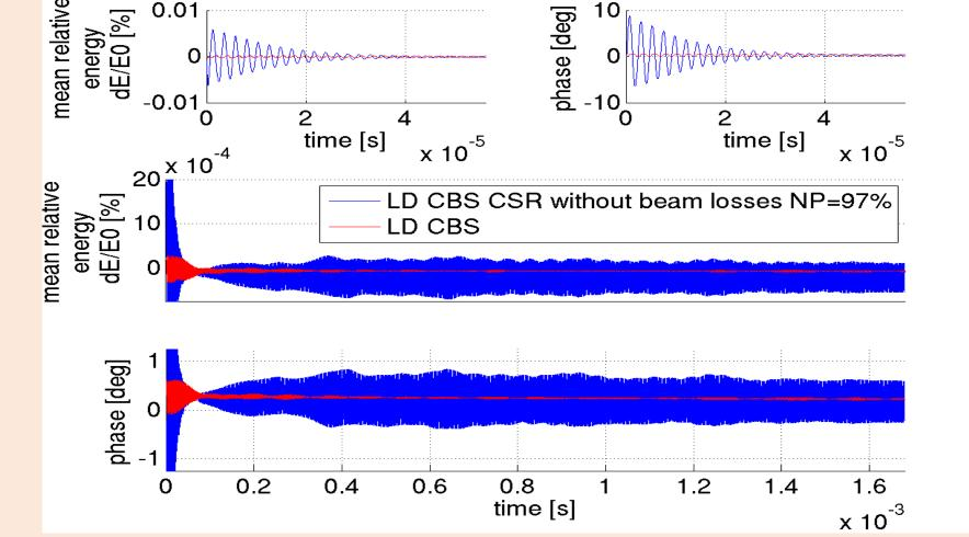
Oscillations of mean relative energy spread (middle) and phase (bottom) of the electron bunch over the total duration of the injection and zoom over the first 50  $\mu$ s (top) with simulation effect of CSR wake field with simulations made without collective effect. NP is number of remaining macroparticles in %
