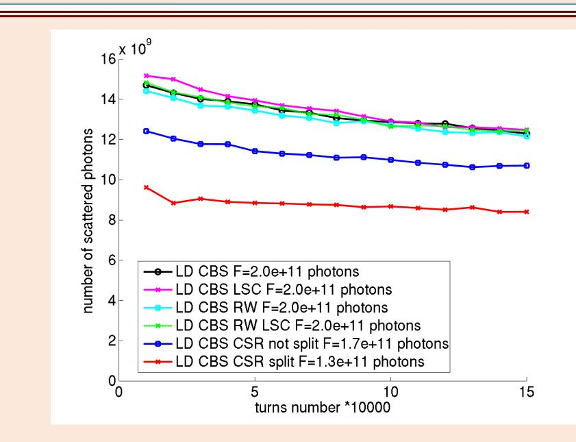
Compton backscattering flux for different beam dynamics effects. In the case of the CSR simulations, if the beam did not split 97% of the particle survived (blue) and 50% survived in the case the beam did split (red). F is the total flux integrated over 150000 turns.
