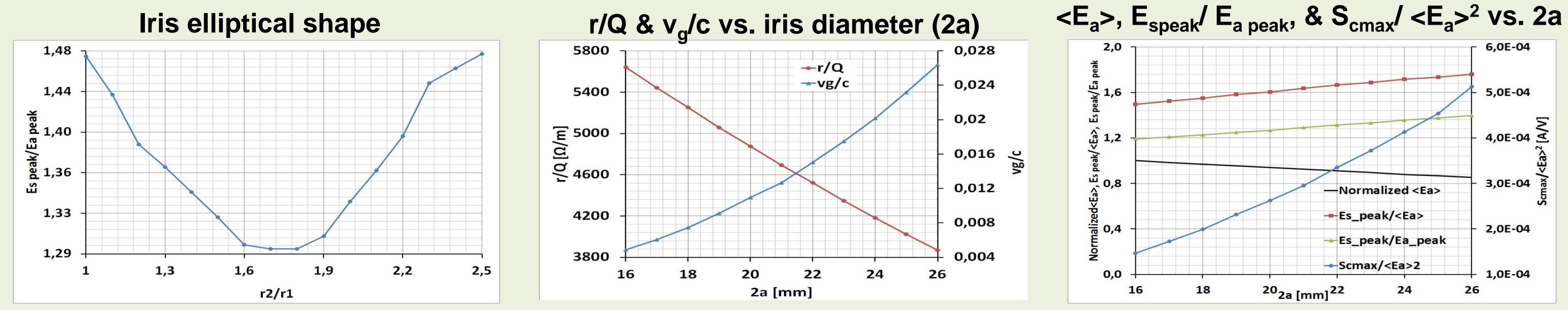
Elliptical iris shape: maximum reduction of r/Q higher for smaller a => reduced wall power diss., the surface field around of 14% compared to v<sub>g</sub> higher for larger a => reduced FT => shorter t<sub>pulse</sub>, smaller a, circular profile.
